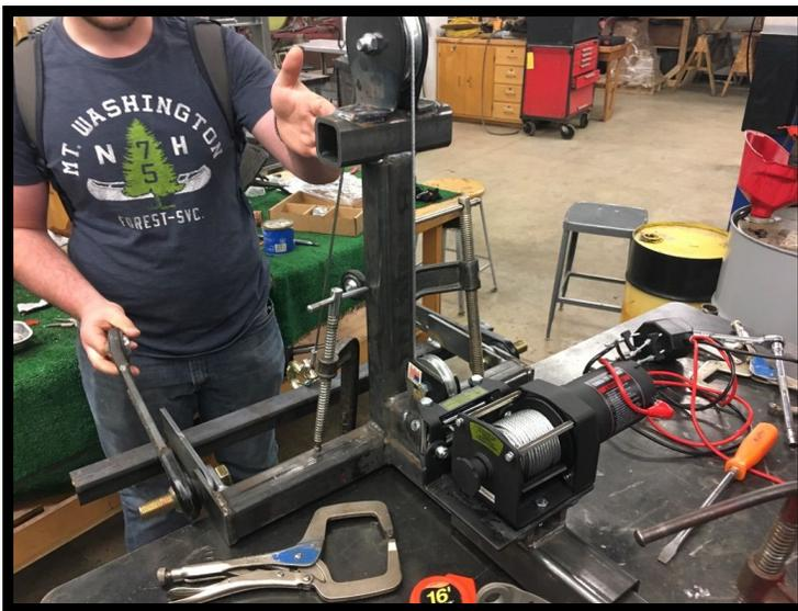
The picture to the left shows the 3-point hitch for our customer's ATV which moved along smoothly. This project allowed us to learn as we completed the hitch and make improvements as we went along to ensure the go. This photo was taken as the winch was attached to the hitch for testing. This allowed the design team to explore options to determine the proper way of securing the winch to the system.
